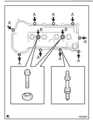
(c) Install the cylinder head cover with the 9 bolts, 2 seal washers and 2 nuts.
