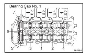
(q) Examine the front marks and numbers, then tighten the bolts in the order shown in the illustration.
