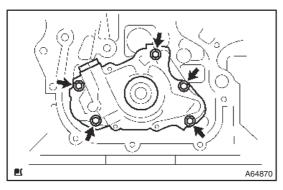
(b) Install the oil pump with the 5 bolts.
