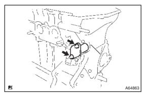
(c) Install the chain tensioner with the 2 nuts.
