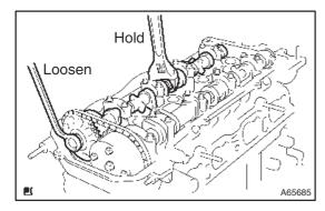
(d) Hold the camshaft with a wrench and so on, then loosen the camshaft timing gear set bolt.
