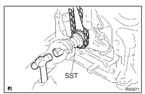
(c) Using SST, install the crankshaft timing gear. SST 09223–22010
