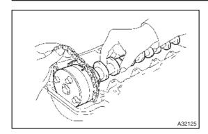
(h) Remove the camshaft while holding the chain.
