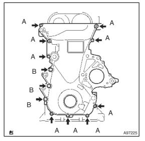
(d) Install the timing chain cover with the 10 bolts and 2 nuts. **Torque:**
