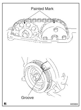
(s) Check the painted marks on the chain and camshaft timing gears, and that the camshaft pulley groove is aligned with the timing mark "0" of the timing chain cover.
