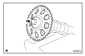
(b) Remove the bolt, then remove the camshaft timing gear or sprocket.
