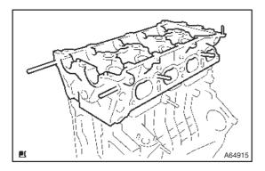
(c) Remove the cylinder head from the cylinder block.
