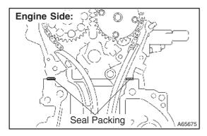
(c) Apply a continuous bead of seal packing (Diameter; 3.5 to 4.5 mm (0.138 to 0.177 in.)) as shown in the illustration. **Seal packing:**
