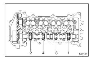
(g) Loosen the bearing cap bolts on the camshaft in the order as shown in the illustration, in several passes, then remove the bearing caps.
