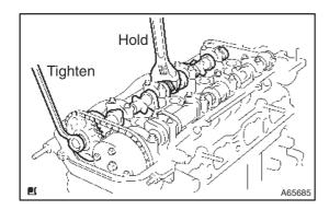
(r) Hold the camshaft with a wrench and so on, then tighten the camshaft timing gear set bolt.
