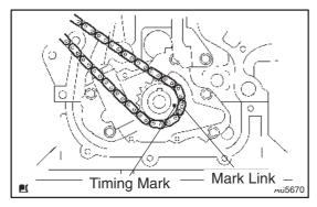
(b) Install the chain onto the crankshaft timing gear with the yellow mark link aligned with the timing mark on the crankshaft timing gear.
