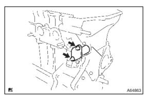
(3) Install the chain tensioner with the 2 nuts.
