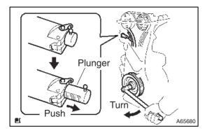
(5) Turn the crankshaft clockwise, then check that the slipper is pushed by the plunger.
