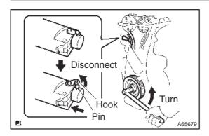
(4) Turn the crankshaft counterclockwise, then disconnect the plunger knock pin from the hook.
