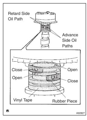
(b) Check that the camshaft timing gear assembly does not rotate.
