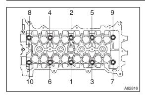
(c) Using a bi-hexagon wrench 10, install and uniformly tighten the 10 cylinder head bolts with plate washers, in several passes, in the sequence shown.
