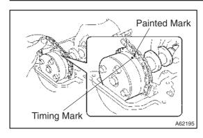
(m) As shown in the illustration, install the chain onto the camshaft timing gear with the painted mark aligned with the timing mark on the camshaft timing gear.
