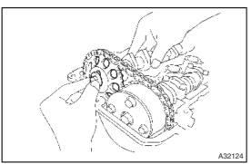
(p) Tighten the set bolt temporarily while raising the camshaft.
