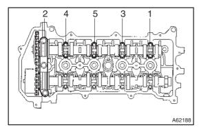
(e) Loosen the bearing cap bolts on the No. 2 camshaft in the order as shown in the illustration, in several passes, then remove the bearing caps.
