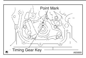
(2) Using a crankshaft pulley bolt, turn the crankshaft to align the timing gear key with the point mark on the oil pump.
