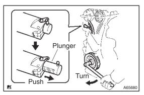
(d) Turn the crankshaft clockwise, then check that the slipper is pushed by the plunger.
