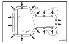
(c) Install the oil pan with the 14 bolts and 2 nuts.
