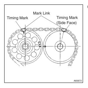
(d) Install the chain onto the camshaft timing gears with the yellow mark links aligned with the timing marks on the camshaft timing gears.
